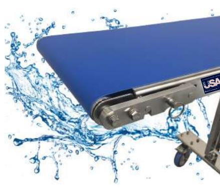
\*Standard belt widths 6" or 12". Standard lengths from 2' to 10'. \*Custom solutions or sizes will require slightly longer lead times.
