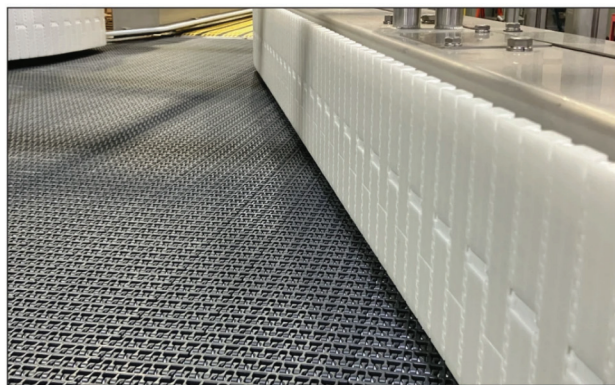
Powered Side Rail Merge Assist. Image courtesy of Multi-Conveyor
