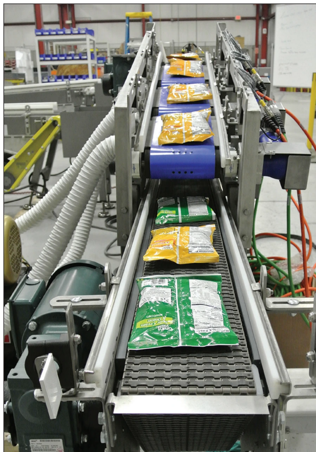
Asynchronous 2:1 Merge. Image courtesy of Multi-Conveyor
