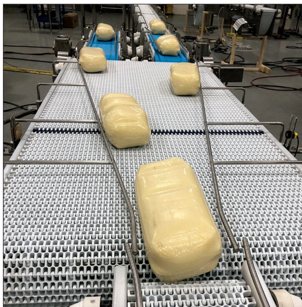
2:1 FIFO Metered Merge. Image courtesy of Multi-Conveyor
