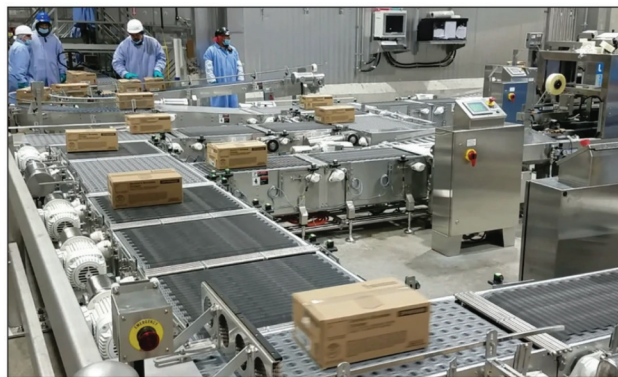
Servo Belt Case Merge. Image courtesy of Multi-Conveyor
