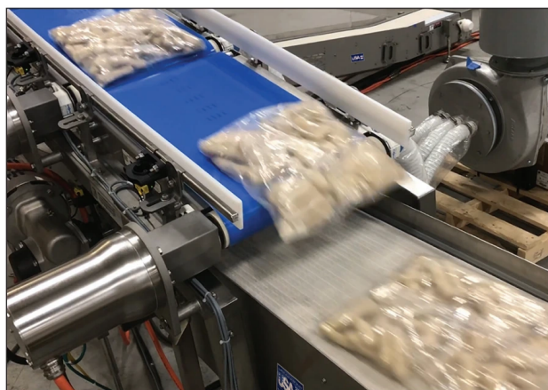
2:1 Vertical Stacked Inject Merge. Image courtesy of Multi-Conveyor
